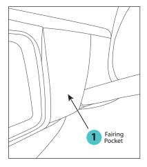
Remove the factory original USB Female Cable from the fairing pocket and replace with the USB Female Cable from the GSR-HM51.
